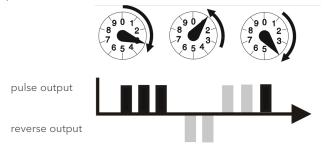
Reverse volume pulses are compensated by identical number of forward pulses before continuing with output pulses.
