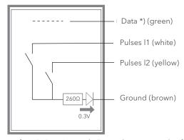
$^{\star}$  active for HRI Data Unit only External power supply of 5 to 24 V DC possible if data line is not used (green)
