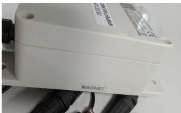
After the magnet is applied, the Radio Module will send the current value of the pulse counter to all ports.
